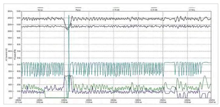
Chart 1: As found, data logging showed undesirable loading and unloading of the base compressor.
