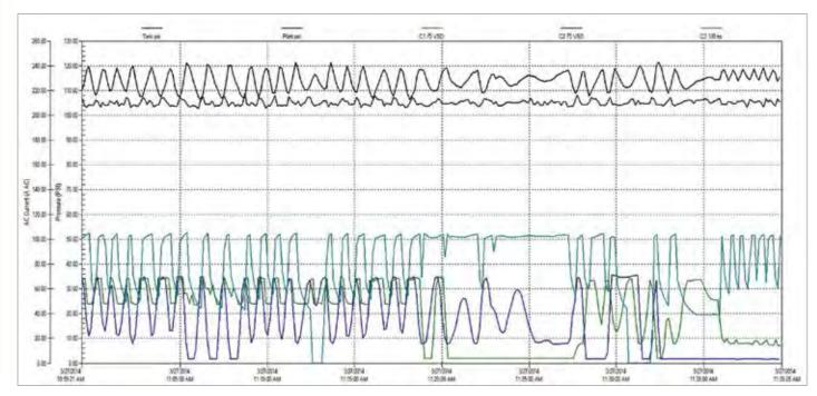
Chart 2: Activating the compressor sequencing controller put the system out of control, making matters worse.
