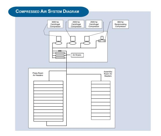
lower. It was possible to lower the compressor discharge pressure settings significantly, and the average main header pressure went from 75 psig to 70 psig. This change not only reduced the amount of energy that was required to produce the compressed air (see text box), but also reduced artificial demand (see text box), which contributed to lower compressed air and energy consumption.
