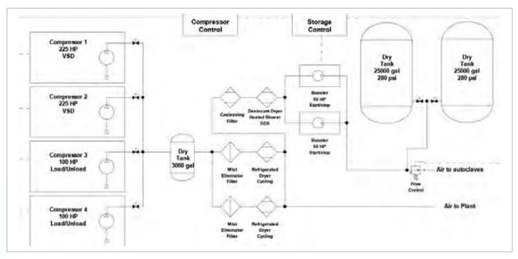
Figure 1: System arrangement uses a high pressure storage
