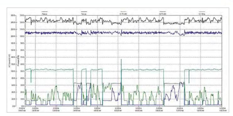
Chart 3: Non-standard local pressure band settings were used to improve compressor control, and the controller was shut down.
